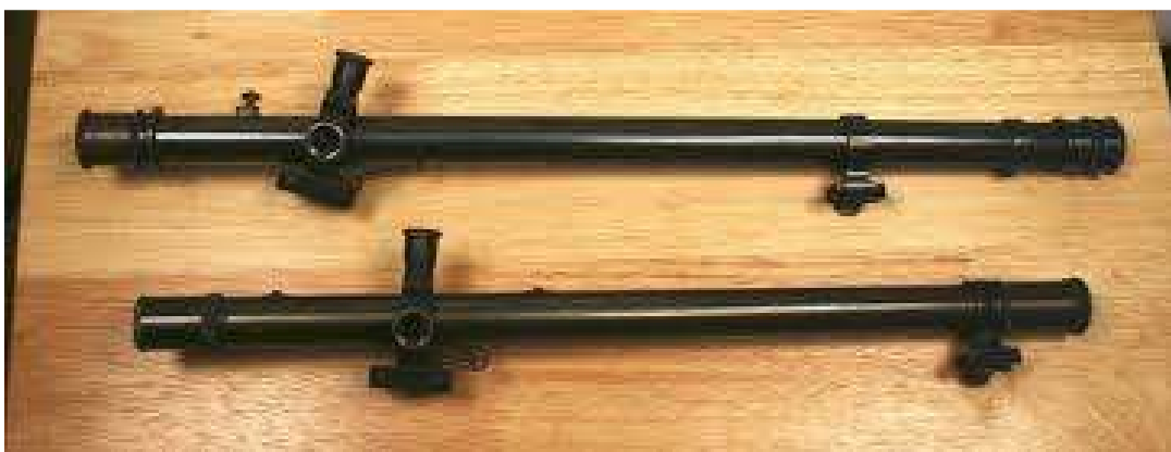
Winchester A5 scope – upper and B3, 4, or 5 scope–lower. Notable is the different overall length. (Author photo)
