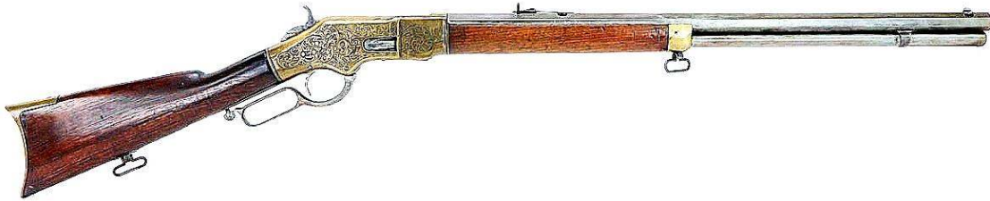
The Model 1866. Finally the design featured a wood forearm, an upgraded gated loading mechanism and a fully enclosed magazine tube. Originally made in .44 rimfire like the Henry -- later issues may be found in caliber 44 Henry or 44WCF (44-40); these were often conversions. Carbines, rifles and muskets were variations. (File photo)
