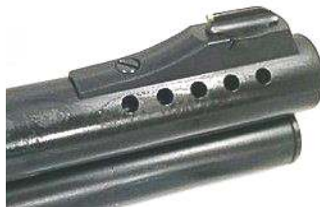
The latest of the Miroku front sight development, this on a .450 Marlin rifle. It shows the typical porting and a new type, bolt-on ramp sight arrangement with no provision for a hood. It is found on the takedown version of the .450 Marlins as well. Previous models/calibers had a dovetail-type front sight. (Author photo)
