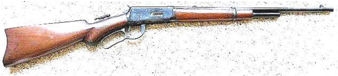
A very rare pistol-gripped, uncheckered, carbine buttplate stock and tang sight on a 2/3rds magazine specimen – the buttstock appears to be slightly dropped as well – nice combination (Author photo).
