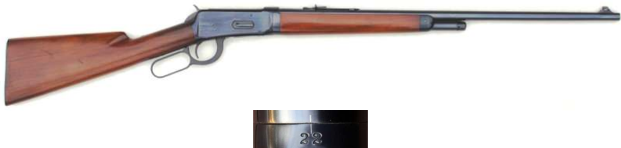
Model 55 serial 22 the finest known original and untouched specimen extant. Note the original takedown indexing marks above the serial number and the fairly deep fluting on the buttstock.
