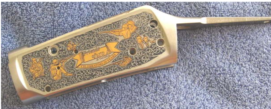
A rare prototype receiver of a “Friends of the N.R.A.” banquet gun. This was likely a take-to-the-boardroom-for-approval example. It has no serial number and is stamped EXP inside the upper tang. Roll or Laser engraving. (Author’s collection)
