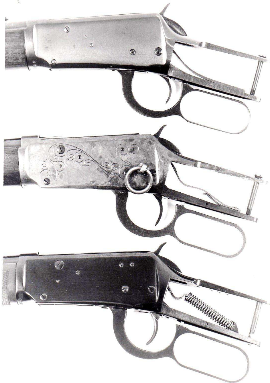
An illustration of the flat mainspring system of the first, second and 2A models (top), the reworked but still flat mainspring of the third and 3A models (middle), and the radical change to a coil type mainspring system introduced on the fourth model (bottom). Note the different placement and the type of screws, pins etc. The coil spring system remained with minor changes throughout the angle eject models to final U.S. production (near serials of 6.6M). (Author photos)
