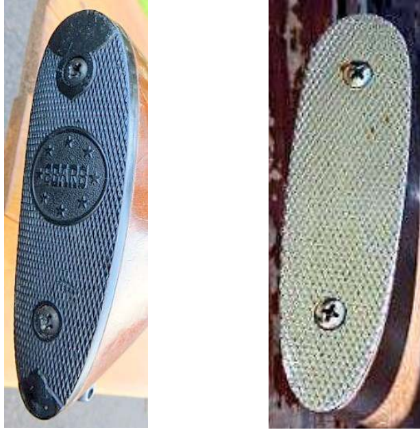
Buttplate design on both Sears models – plastic/hard rubber (left). Some examples had typical Winchester flat-checked buttplates and some of these are nickel plated (right). (Author photos)
