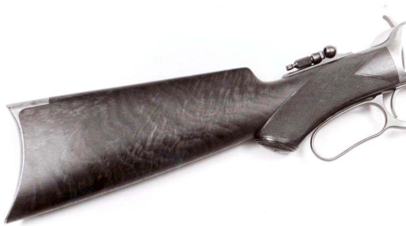
A superlative example of a high grade walnut, pistol-gripped deluxe rifle buttstock with Style "H" checkering; tang marked XX. (Author photo)
