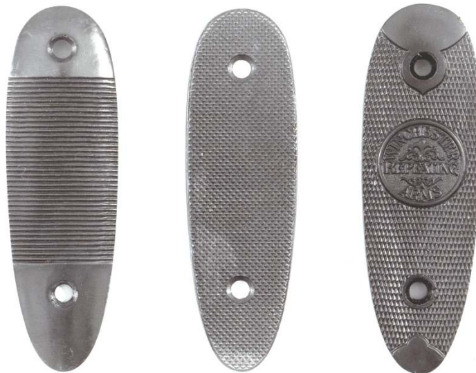
Again, left to right. Model 55 style serrated steel used on prewar Model 94 carbines as well as the Model 55. The flat checkered steel (later phenolic) buttplate, in use until the late 1970s and starting as standard in the postwar period (1946) but they have been seen (very sporadically) in the earliest 40s – note the revised screw locations. Checkered hard rubber 4-3/4-inch shotgun style with logos; seen on standard guns through the end of production – the logo and slight cosmetic changes of this type coincide with corporate changes. (Klein photo)
