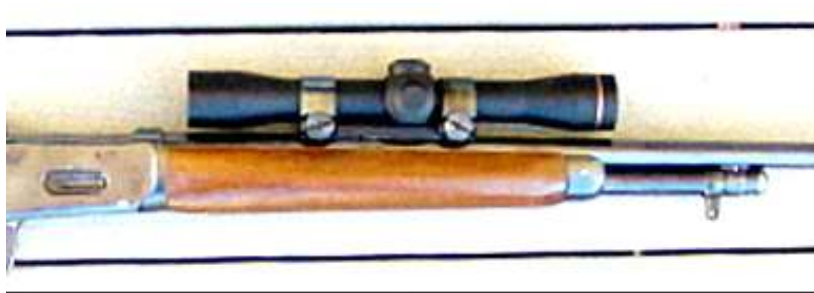
A very scarce scout style mounting with the ever-popular Leupold M8-2X scope on a standard Model 64. This is the only example I have seen and it requires more gunsmithing than the same style mounting on a Model 94 carbine. It also leaves the host gun with at least one extra hole drilled into the barrel itself. A neatly accomplished and useful undertaking. (File photo)
