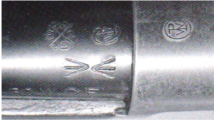
This is a Canadian proof/acceptance marking sometimes found on the barrels of Dominion of Canada Model 1894 carbines. Less than 30 are known at this time. (Author photo)
