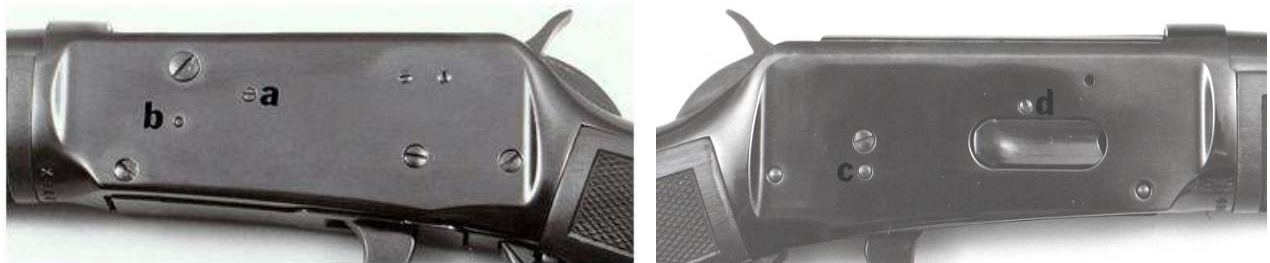
The third, 3A and fourth model external receiver detail. On the left side (upper) we see that the cartridge guide screw (A) is again installed from the outside (a Type 3 to 3A change). The end of the carrier spring screw (B) is now visible between the bolt/lever pin stop screw (larger head diameter than before) and the link screw. On the lower example (right side) we can see the end of the (now through design) carrier screw (C) just below the loading gate retaining screw, the head of which is seen in a corresponding location on the left side. The right side cartridge guide screw (D) is visible above the loading port and is also installed from the outside. The loading port cover (on Type 4s) no longer has the two-piece look of Type 3 or some 3As. (Author photo)
