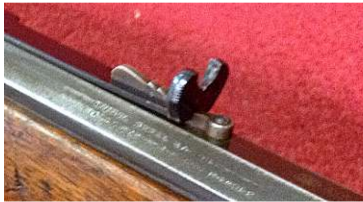
A rarely seen 32B type elevator with a screw installed where the thumbpiece would usually be, for “finer tuning.” (Author photo)
