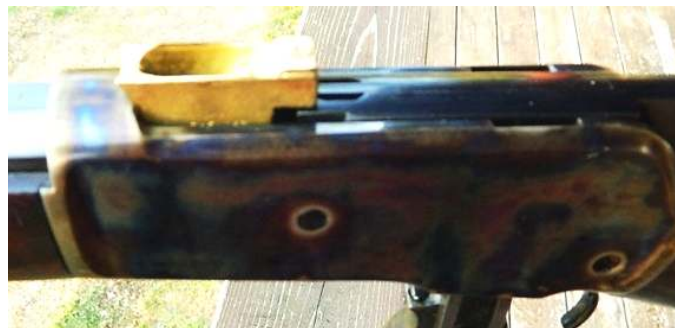
This is a neat and very scarce item. A Winchester-made bore mirror. The method of use is obvious and YES, I know a Model 92 is shown. The unit is not model or even brand specific and is applicable for use with all Winchester lever-action models and many other brands/models as well. (Author photo)
