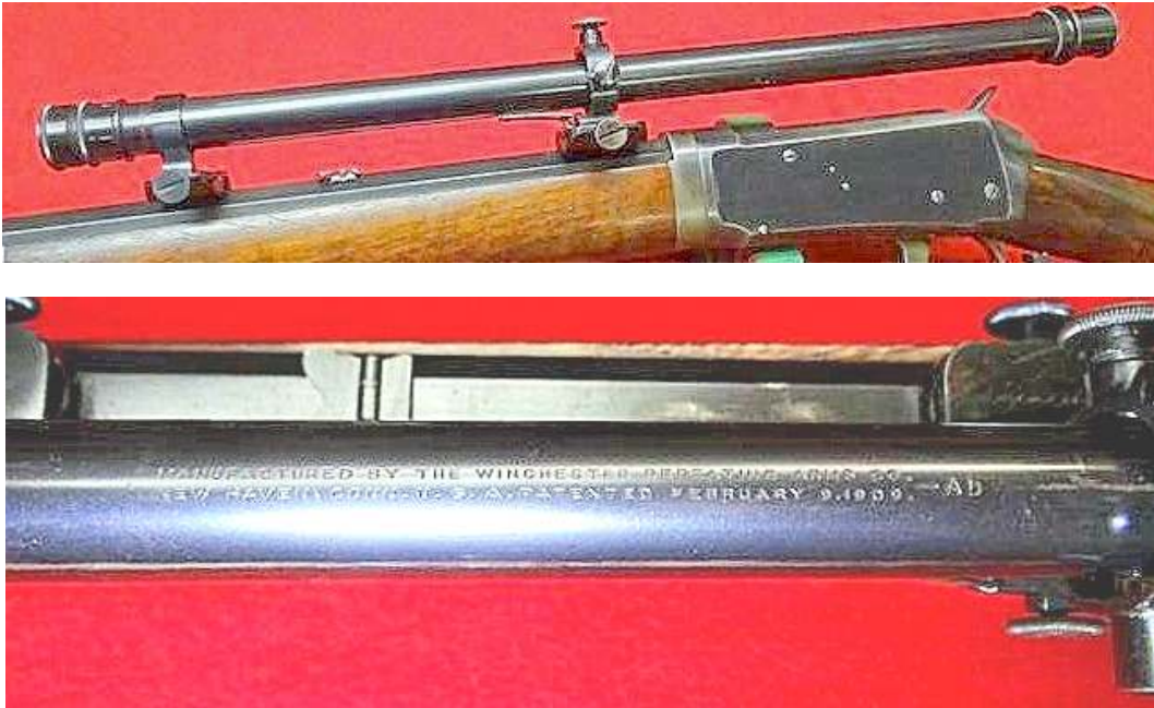
A factory installed A5 scope – Bennet mounting. Notice the very rare offset mounts. Also notice the correct thumbscrews that would lock into the mount. This specimen has the offset proofmark to the left tending to indicate factory assembly. (Author photo)
