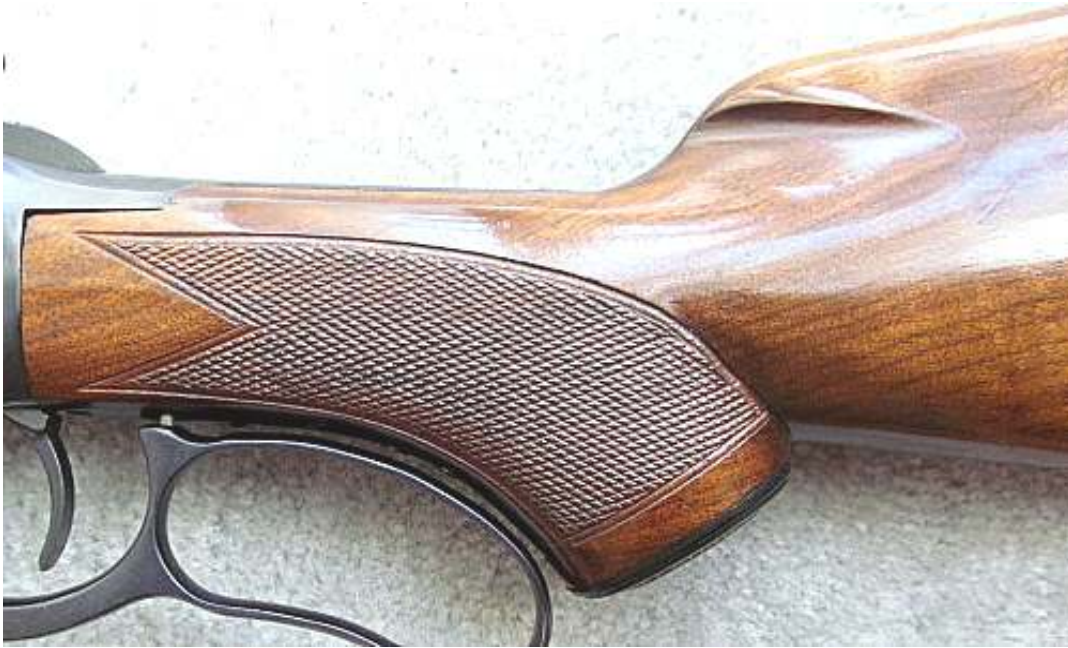
Late model coarse checkering (18 LPI or evenless) on a thicker pistol grip with a larger gripcap. Note the more aggressive Whelen flutes and some mistakes in the checkering and final fit that likely would have been rejected earlier in the Model 64s production era. Speculation is that this may be a Model 71 stock, modified and fitted to a Model 64 very late in production – NOTE: speculation . (Author photo)
