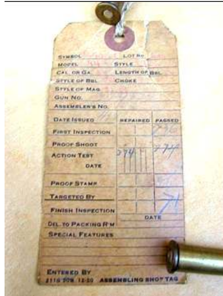
Details regarding the inspector's tag on the specimen below – one serial numbered and tied to each gun. Very difficult to read – after all, it is from the 1920s. (Author photo)
