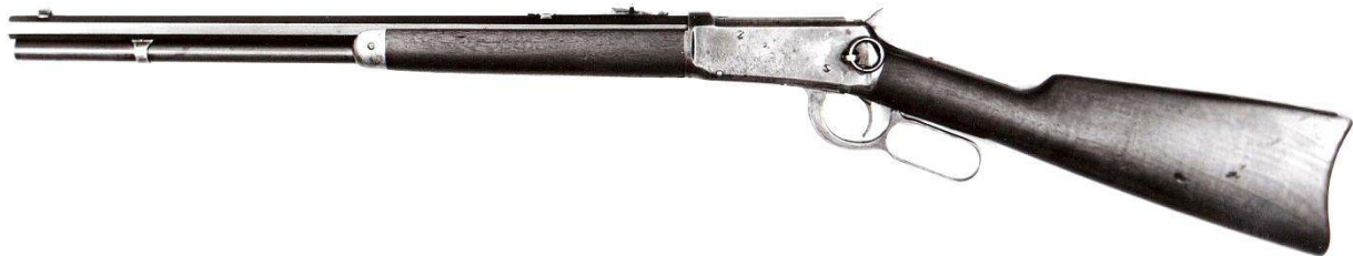
A very scarce example of a 20-inch octagonal barreled short rifle with both a saddlery and a carbine buttstock. Likely special ordered to have a carbine sized gun with a little more "heft" than a standard carbine. Note the shorter 8-1/2-inch forend and the 4-inch rear sight location. (Author photo)
