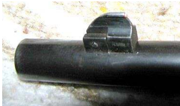
A popular but still fairly scarce Marbles number 94C front sight enhancement accessory. It replaces the simple blade with an extension having a gold or ivory bead. There were several optional sizes (blade heights) to tailor the sight to the caliber of the gun or the taper of the barrel. These were also available from Sheard and likely others. They sold for about $1 "back in the day." (Author photo)
