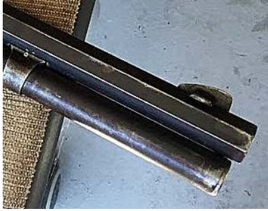
The Rocky Mountain sight mounted in the reversed position – not often seen. On the right is a small hand-made rocky mountain type, likely made from a small piece of brass or a coin. (Author photos)
