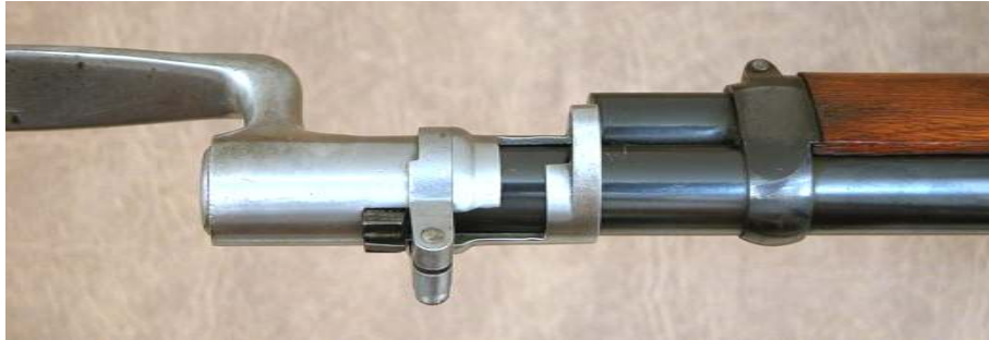
The bayonet mounting detail – Serial 503008, 1909 --30WCF, 30-inch barrel – note the front band; not really a cap. (Rob Kassab collection and photos)
