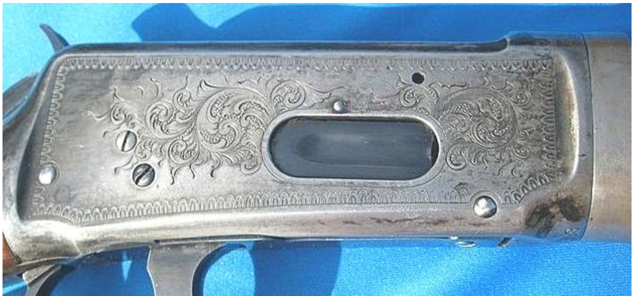
A decent example of what appears as non-factory engraving. Non-factory work is very likely and is noted by the mistakes in the bordering above and below the loading port. More of these exist by far than originals but many easily surpass the quality of factory work. They nonetheless are not regarded “as valuable” as an original factory ordered specimen unless perhaps when signed by a renowned and respected, non-factory engraver. As commonly seen with Colts, I suspect that many Winchester models were relegated to outside contractors for embellishment prior to retail shipping. (Author photo)
