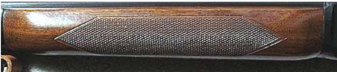
A Post war through the end of Pre-64 production, coarsely checkered (18 LPI) forend, with an obviously larger panel. The checkering seen here is also sub-par – note the bordering. As mentioned earlier, this change in the checkering specification is due to the lower quality (softer) walnut that was procured from eastern sources after WW II. (Author photo)
