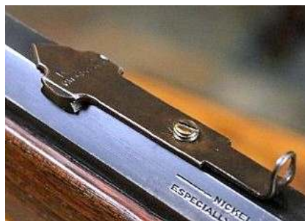
A King manufactured "ghost ring" or "loop" styled rear sight (patented 1933) complete with an elevation adjustment screw. (Author photo)
