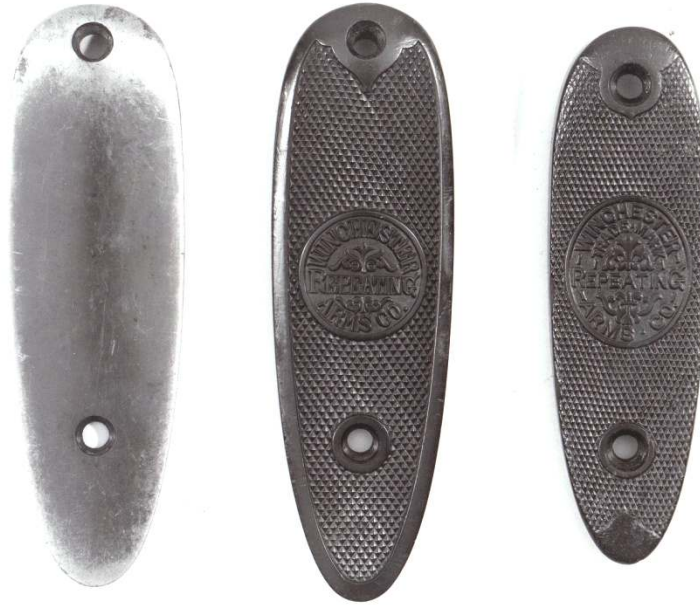
Some “standard” buttplates. From left to right – Smooth steel shotgun style with no rollover or “widows peak;” these are most often found with the widows peak – checkered hard rubber, 5-inch shotgun style with logo – 4-1/2-inch checkered hard rubber shotgun style with logo, used on some prewar carbines. (Klein photo)
