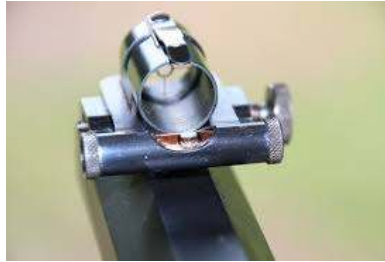
A very fine windgage/spirit level sight with a circle-crosshair-style aperture. (Author photo)
