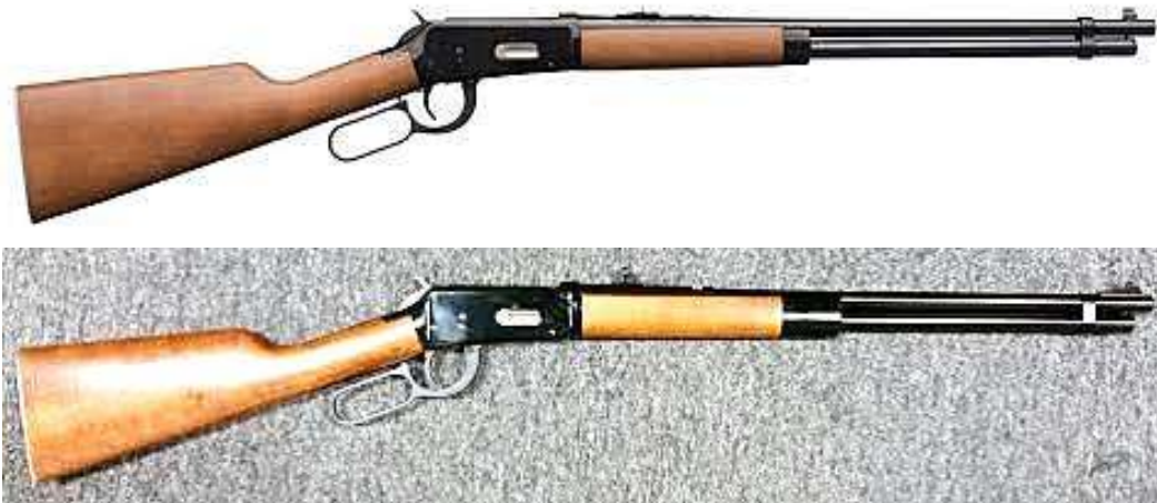
The upper illustration is of the lesser quality hardwood-stocked version and the lower is of the higher grade ramp-sighted model with sapwood walnut stocking (on some), a longer forend cap, a ramp front sight and a nickel plated Winchester Model 94 buttplate; note that both examples have nickel plated loading gates. Clearly illustrated is the appearance of identical forend wood length and the differing front sights and bands. The long-forend-cap version has better finish as well. (Author photos)
