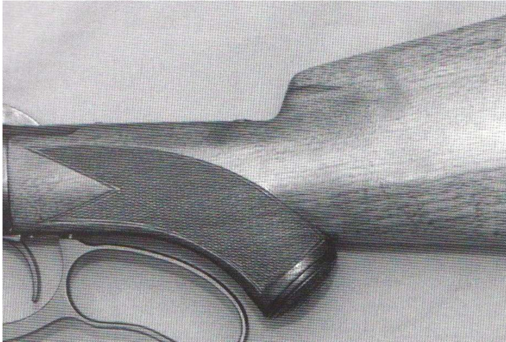
Prewar fine checkering (20 LPI) with a smaller pistol grip and gripcap. Note it is also quartersawn and has a very subdued “Whelen” flute. Also be aware of the quality of the checkering execution. (Author photo)
