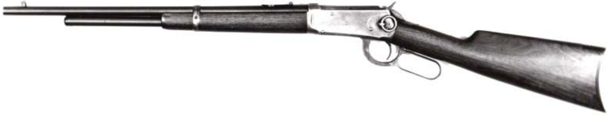
A very rare specimen is this caliber, 32-40, carbine with a 3/4 magazine, an express rear sight and a rifle buttstock. (Author's collection)
