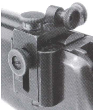
On the left is the Lyman model 56 receiver mounted sight (to about 1953) supplanted with the Lyman 66-A code or later 66A (no code) after that, and on the right is the very desirable Winchester Type 98A bolt mounted peep sight. The Type 98A was available on several Winchester models but is most often seen on the Model 64 in caliber .219 Zipper. (Author photos)
