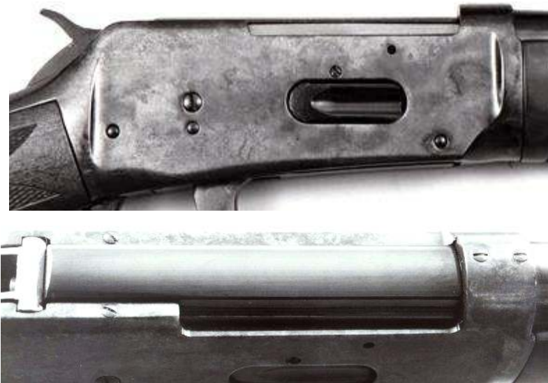
The Type 6 receiver. You can readily identify the clearance cut on the receiver itself, the new bolt design and the repositioning of the extractor. Also visible are the slightly flattened upper frame rails and the screw holes that allow the top mounting of a telescope. On this receiver design just before the 6A at serials of about 5.4-5.5M, and approximately coincidental with the introduction of the drilled hammer, the lower link through-screw reverted back to a pin held in place by a screw through the bottom of the link itself as on the Pre-64s. Note as well the less-than-acceptable modern version of case-coloring.
