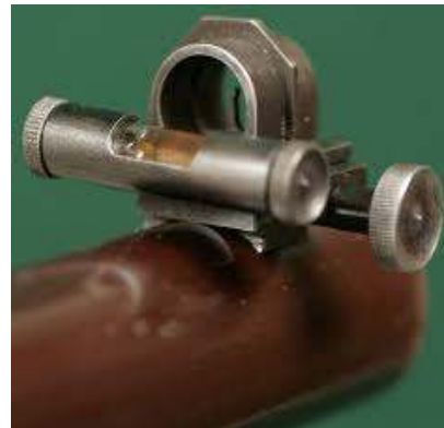
The left illustration shows the "spirit level" sight (with a broken glass tube) and without the windgage base. On the right is the spirit level sight mounted on the windgage base, both can be considered very rare and are most often found on rifles used for precision shooting. They have been verified as originally equipped on highly optioned Model 1894s, and especially 1885s, usually in calibers 32-40 or 38-55; these two calibers are noted to be inherently accurate. (Author photos)
