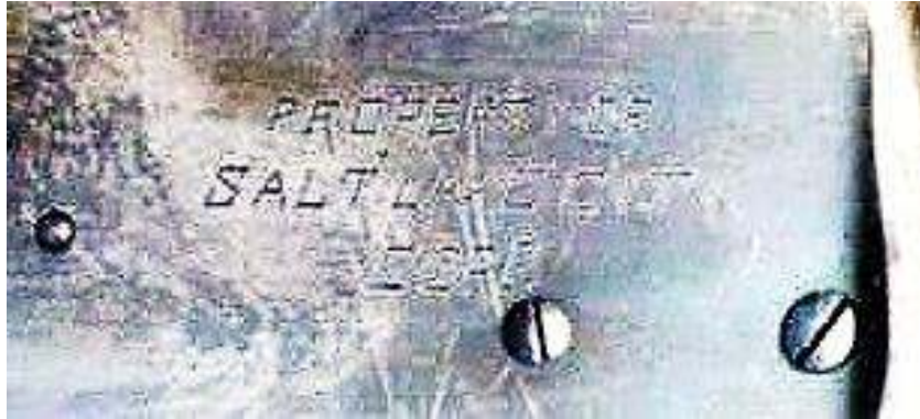
Another non-factory agency marking, Salt Lake City. Crude and not likely factory applied even if a substantial number of guns were contracted for sale to the City. (Author photo)
