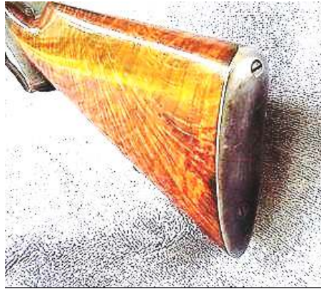
A scarce smooth steel buttplate with a pointed rollover (widows peak). This example showing a nicely feather grained buttstock with pistol grip as well. (Author photo)
