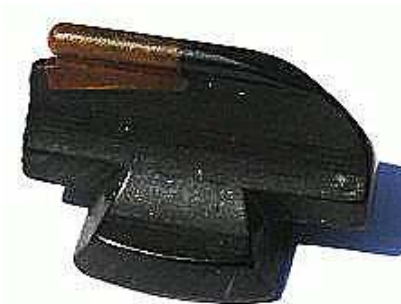
A nicely done brass insert for a blade type front sight. (Author photo)
