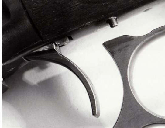
Trigger/hammer/lever safety plunger – typical. See above illustrations for more details. (Author photo)
