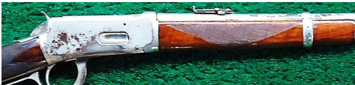
A typical dull and flaked original full-nickel deluxe carbine. Early nickel plating did not have the brighteners used in today's formulas and soon dulled (and flaked) with use – period examples from all manufacturers commonly show this trait. (Merz photo)
