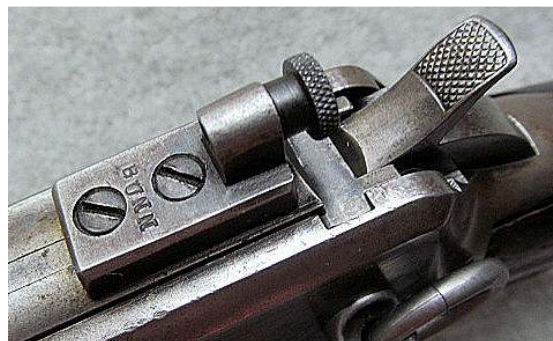
A very scarce example of the “economy,” non-adjustable other than aperture size, Bunn – bolt mounted peep sight. This is one of the better of the many inexpensive examples – all require some gunsmithing and position adjustment. (Author photo)
