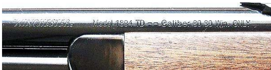
Left side barrel marking (typical) – Japan. Note that they now specify Takedown (TD) but not angle eject (angle eject is now called “countersunk receiver” in Miroku speak). Also visible is the return to Model “1894” instead of the Model “94.” Note the “lawyer” marking (“ ONLY ”) after the caliber designation. (Author photo)
